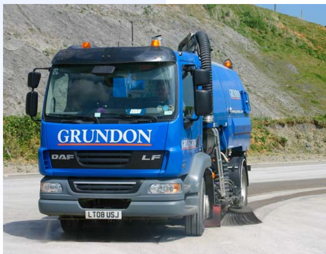
Sweeper vehicle with low emission EURO V engine
