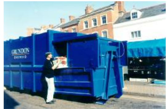
Large mobile compactor
