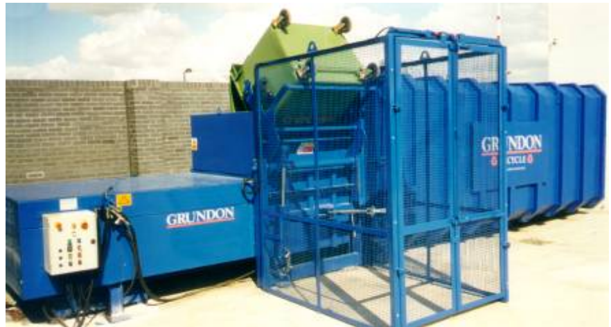
Static compactor with hydraulic tipping of Grundon Waste Wheeler containers
